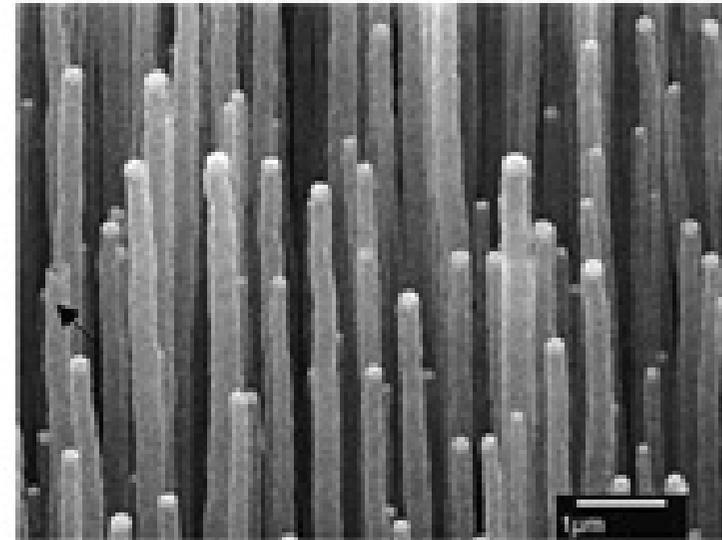
A nickel cap is on the tip of each nanotube (except arrow).
