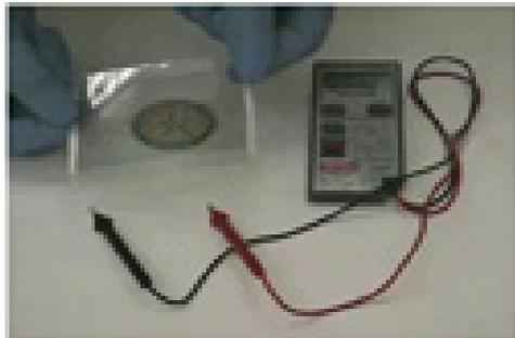
When sandwiched between plastic sheets, MWNT sheets can be bent with no change in electrical conductivity; this is important for flexible electronic circuits.
