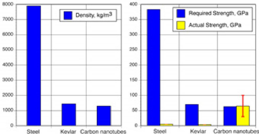
The carbon nanotube strength value depends on the number of defects assumed.
